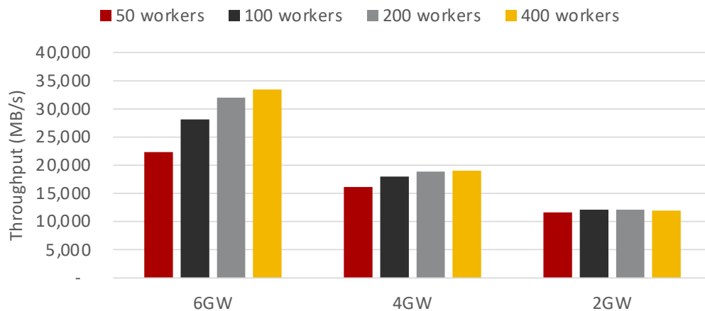
S3 Data Services Node Scaling - READ
